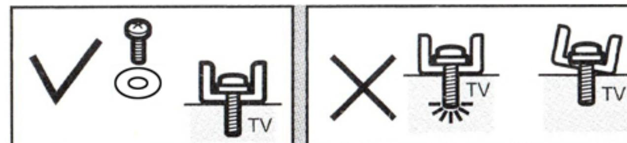
Select appropriate screws to connect the hooks to the TV. If the horizontal and safety screws on the top and bottom of the hooks block the installation holes, you can first remove the blocked screws. After connecting the hooks to the TV, reinstall the removed screws.
