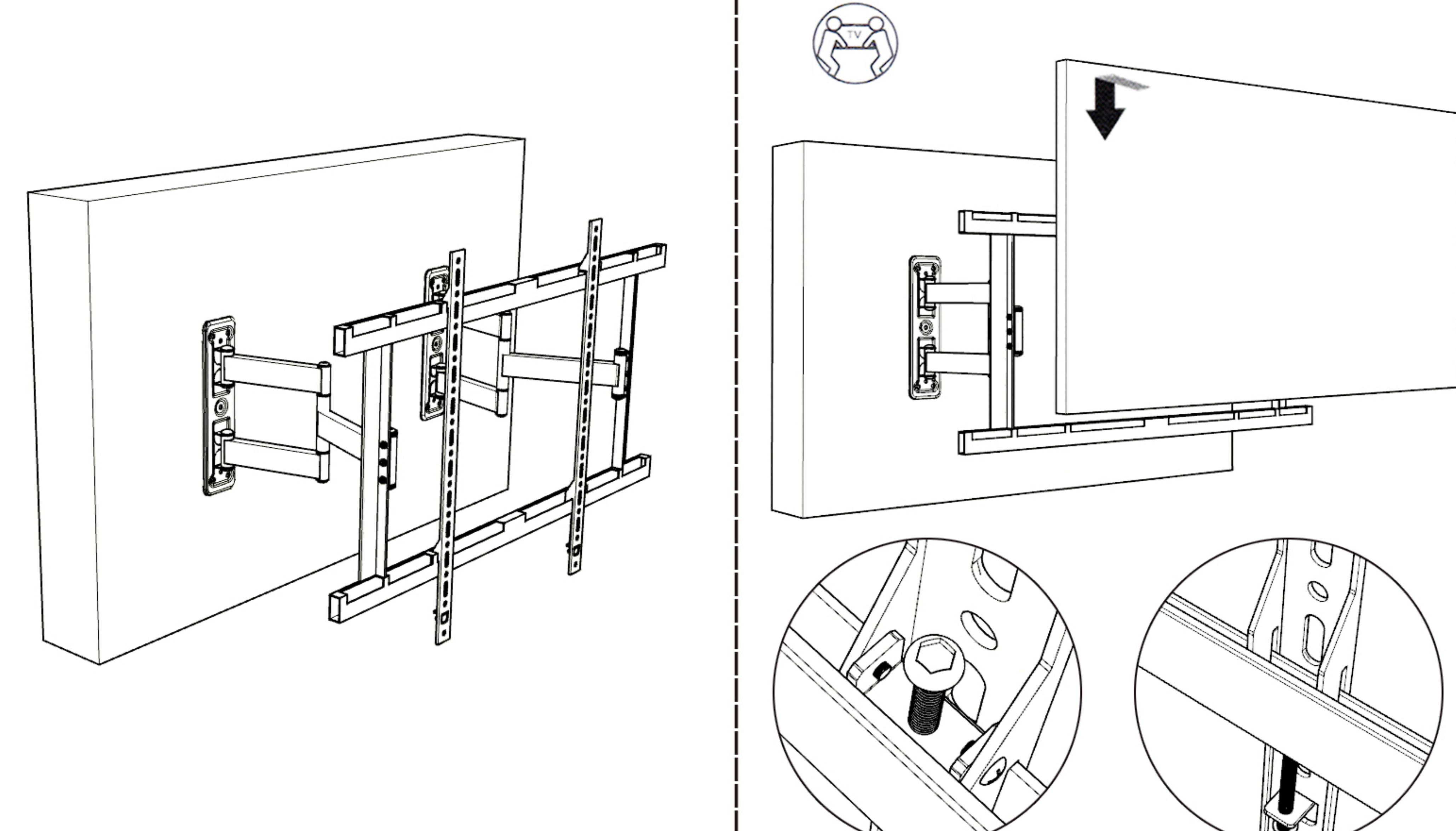
First, pull out the TV bracket and then hang the TV hooks into the open slots of the crossbeam.
